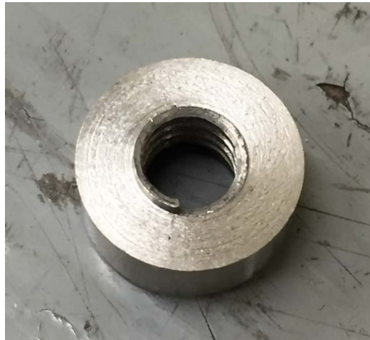
Figure 4.1: Plain stainless steel sample to be used in experiments.
