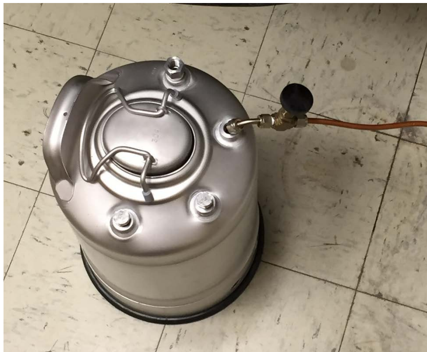
Figure 3.4: Waste fuel reservoir.
