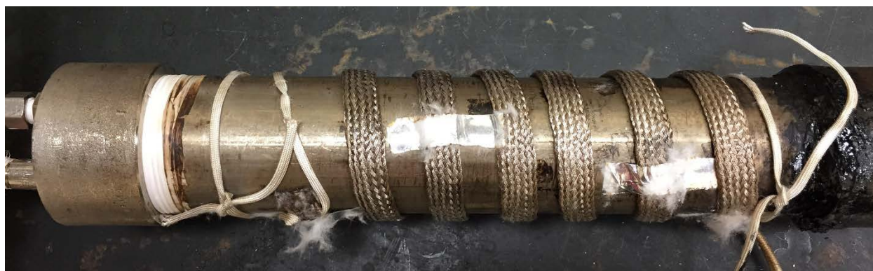
Figure 4.2: Testing chamber with heat cable installed.
