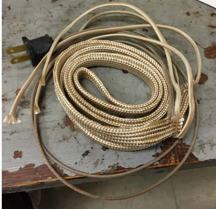
Figure 3.5: 313 Watt heat cable with 120VAC plug.
