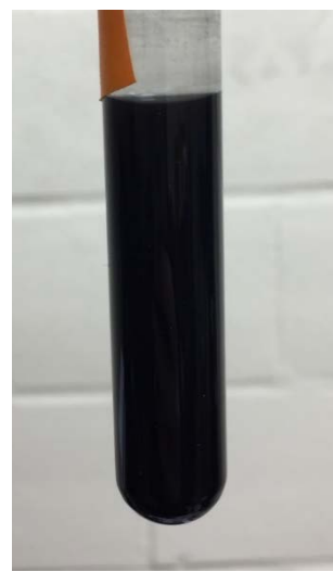
Figure 4.6: Jet-A with 0.1% CNP, 1.5% surfactant. 30 minutes after mixing.
