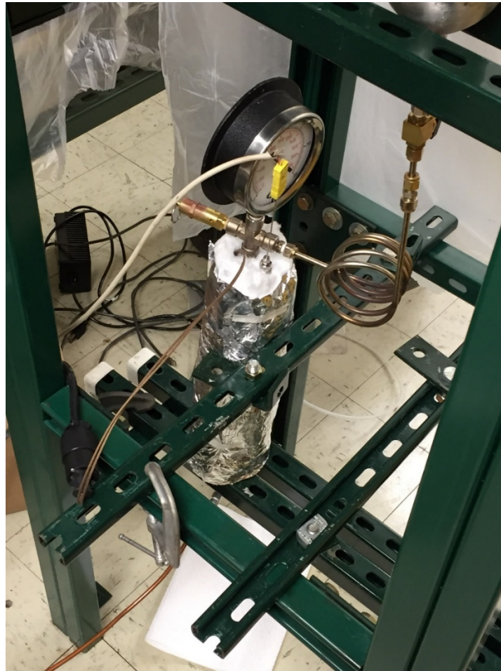
Figure 4.3: Fully insulated testing chamber connected to the pre-heated vessel and waste reservoir.
